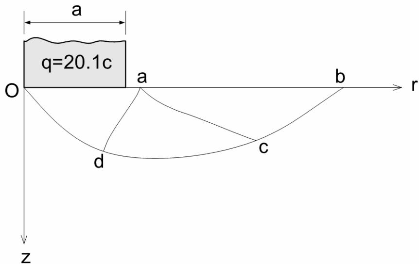
Figure 1. Cox slip-line net for a smooth circular footing where  $q$  is the bearing capacity (20.1 times the cohesion).  $Z$  is the axis of symmetry.
