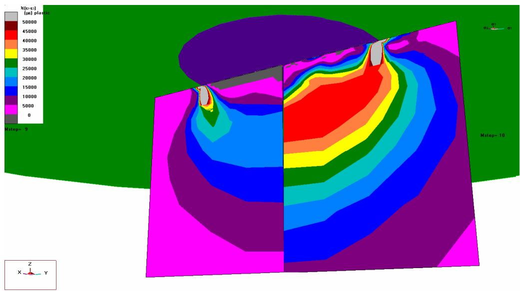
Figure 6. Contours of plastic strain beneath the circular footing prior (LHS), and at (RHS), the bearing capacity for MS9 and MS10 respectively.
