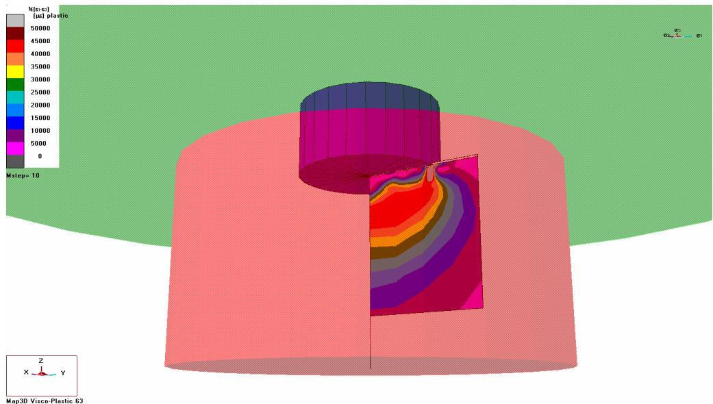
Figure 5. Contours of plastic strain beneath the circular footing at the bearing capacity (MS10). Hidden geometry is shown as translucent.
