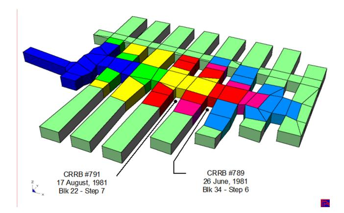
Stresses are calculated at the centre of each of the observed pillar failures at the point in the sequence when the failure occurred.
