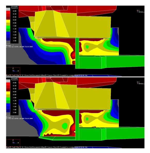
Below are shown the strength factor for the high estimate defined as  $\{\sigma_3 + (m \times \sigma_{c50} \times \sigma_3 + s \times \sigma_{c50}^2)^{\frac{1}{2}}\}/\sigma_1$  at Step #3 and Step #4.
