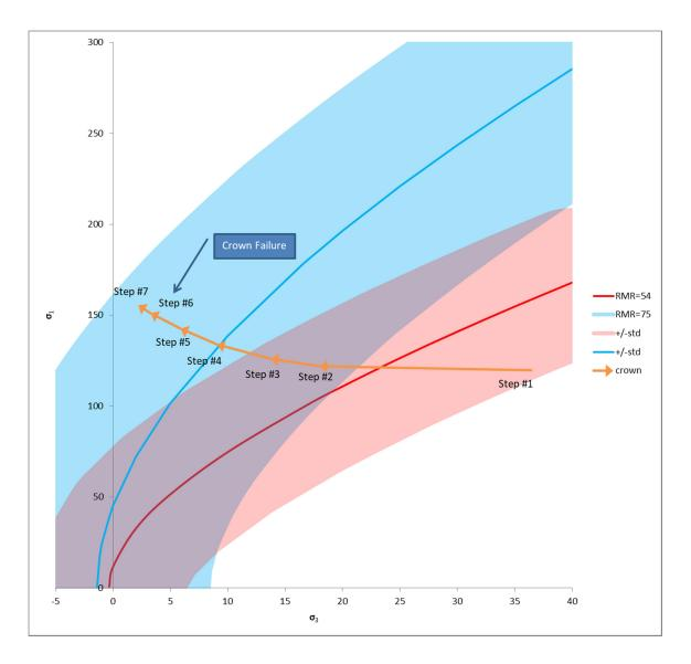
The Hoek-Brown low estimate gives an expected failure of the crown pillar sometime between step #1 and step #2 with a 1 standard deviation uncertainty (confidence interval between 25% and 75% probability) of about 1 to 2 steps (years). A 2 standard deviation uncertainty (confidence interval between 5% and 95% probability) would give an uncertainty that encompassed the entire pillar width.
