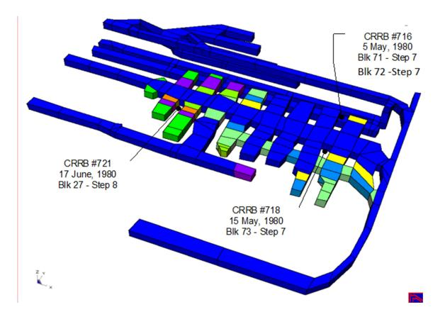
Stresses are calculated at the centre of each of the observed pillar failures at the point in the sequence when the failure occurred.
