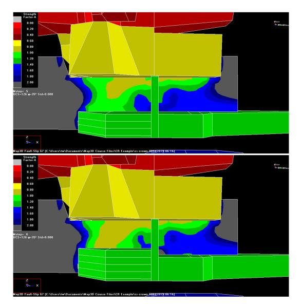
Below are shown the strength factor defined as (UCS +  $q \times \sigma_3$ ) /  $\sigma_1$  at Step #5 and Step #6.
