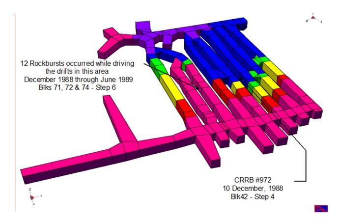
Stresses are calculated at the centre of each of the observed pillar failures at the point in the sequence when the failure occurred.
