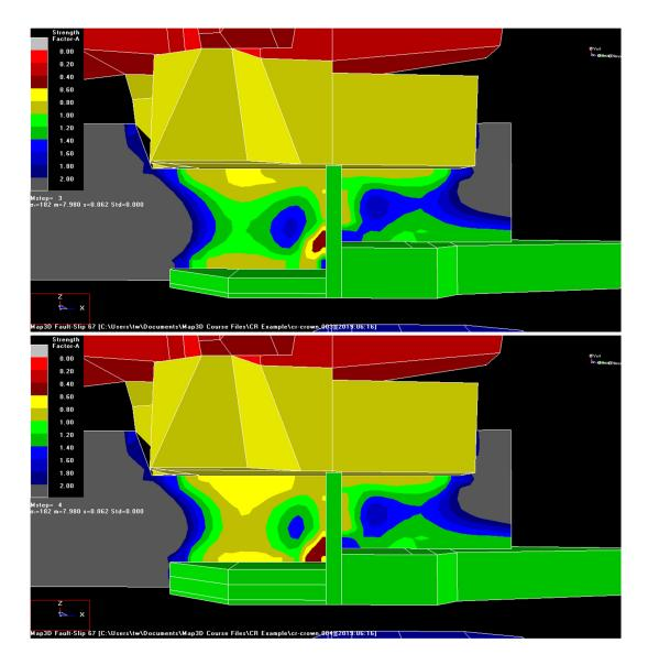
Now consider a failure prediction made from the calibration for the silling out on 6800, 7000 and 7200 levels (blue diamonds below).
