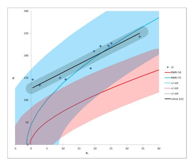
Note that the ±1 standard deviation zone shown corresponds to a confidence interval between 25% and 75% probability. For design purposes, it is more common to use ±2 standard deviation zone which corresponds to a confidence interval between 5% and 95% probability.
