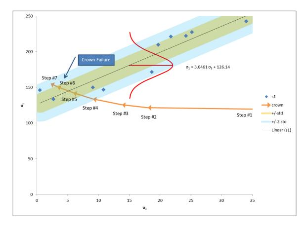
The best fit line through the calibration points is shown in black. This line corresponds to a Mohr-Coulomb criterion with an intercept UCS=126 and slope q=3.65. The fiction angle can be calculated as 35° from the relation  $q = tan^2(45 + \varphi/2)$ .
