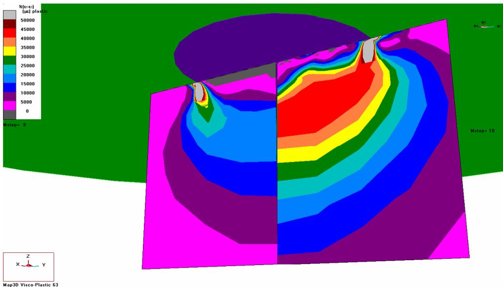
Figure 6. Contours of plastic strain beneath the circular footing prior (LHS), and at (RHS), the bearing capacity for MS9 and MS10 respectively.
