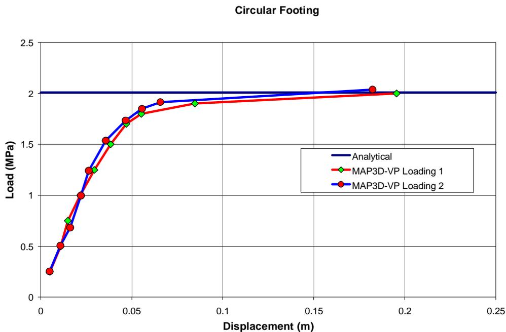
Figure 3. Load vs. displacement response for a circular footing on a Mohr-Coulomb material (includes two different loading paths for comparison).
