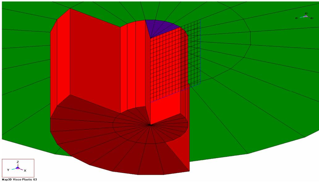
Figure 2. The MAP3D-VP model geometry used for this problem.
