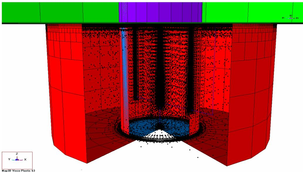
Figure 3. The MAP3D-VP model geometry showing interior nodes.
